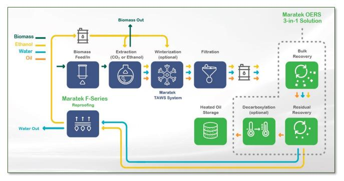
Maratek equipment decreases processing time, simplifies process flow, and integrates the key production steps all to one piece of equipment. These three key production steps are fully automated and controlled by the Maratek control system, fully developed tested and supported, in house.
