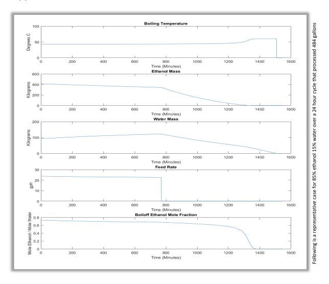
Maratek flow rate guarantees are based on highly reliable data generated by taking into consideration all process parameters including feed solution ethanol/water/oil content, the evolving composition of the still over time, and reduction in boiling power at the end of the cycle to give our clients certainty in our performance specifications.
